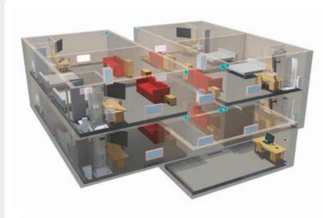
Wireless signals between the gateway and each zones thermostats and radiators are at 433 MHz.
